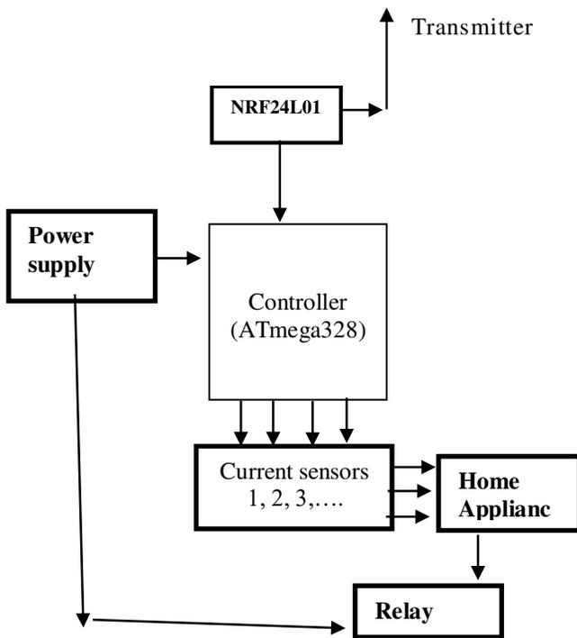
Fig 2. Block diagram of first module
